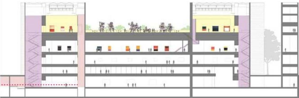
**BUILDING SECTION:** after construction, the upper levels provide 12,000+ SF of new gallery space within the existing building footprint, the enlivened sculpture terrace connects the towers, and every level of the gallery is connected by the new egress stairs
